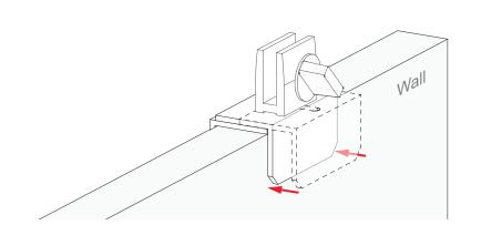
(3) Tighten hex screw to secure Bracket in place.
