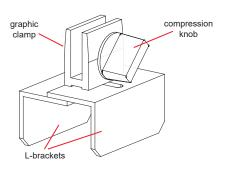
Each graphic panel is supported by two mounting brackets.
